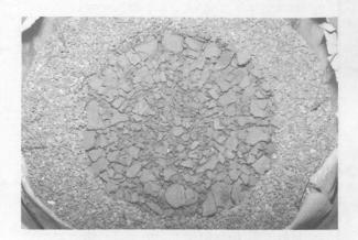
CLEARLY VISIBLE is the contrast in particle size between inner and outer oil shale zones of a lab-scale experiment designed to demonstrate feasibility of Sandia's "second-generation" retorting concept. Experiment used 200 pounds of shale in a 3-ft.-tall test vessel. Although the 8-in.-diam. inner section had a much lower void than the outer region — 25 percent vs. 44 percent — retort and combustion fronts progressed uniformly during the experiment. The MWX
